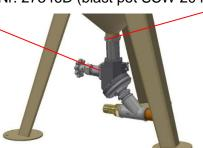
2. Tighten lock nut against threaded sleeve on the blast pot.
