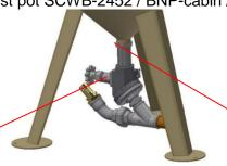
Screw the dosing valve into the blast pot.
